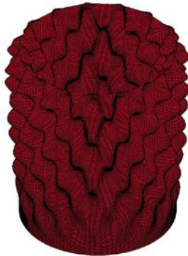
Figure 19.6a - First eigenmode with the 1000 lbf load applied for the six refined mesh discretizations (elform=16) - no contouring.
