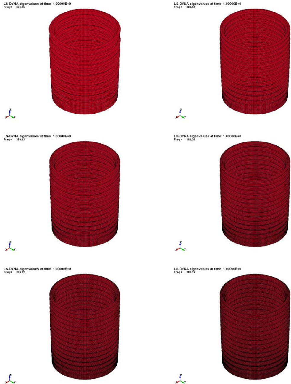
Figure 19.5a - First eigenmode with the 1000 lbf load applied for the six refined mesh discretizations (elform=10) - no contouring.
