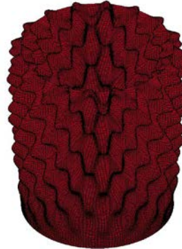
Figure 19.6a - First eigenmode with the 1000 lbf load applied for the six refined mesh discretizations (elform=16) - no contouring.
